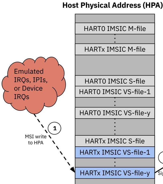
**Example:** Wake-up Guest\_A VCPU\_B from WFI using IMSIC VS-files on HARTx
