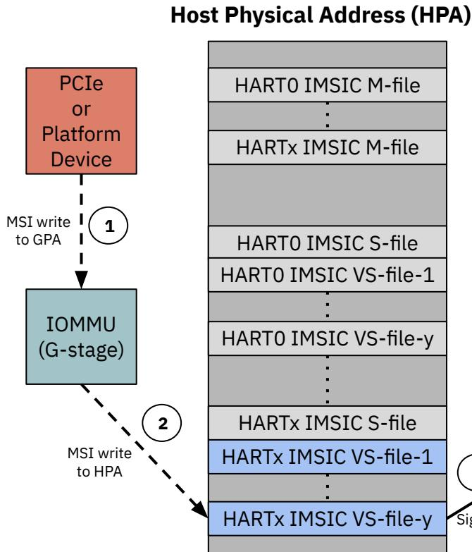
**Example:** MSI from PCIe (or Platform) device targeting Guest\_A VCPU\_B using IMSIC VS-files on HARTx
