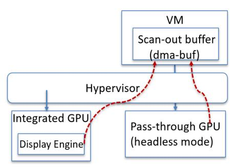
Share guest scan-out buffer between pass-through GPU & integrated GPU
